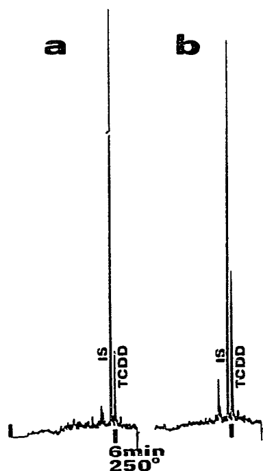
Fig. 2. example of analysis results showing recovery of added TCDD (a) 3.8 ppt recovered; (b) 5.0 ppt added, 9.0 ppt recovered. Column, 20 m \times 0.4 mm I.D. FFAP.
